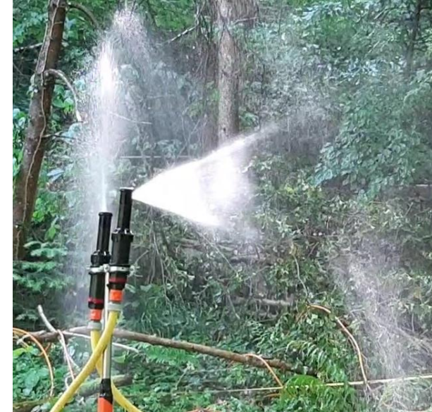
Sprinkled with ~16 mm/h for >3h
