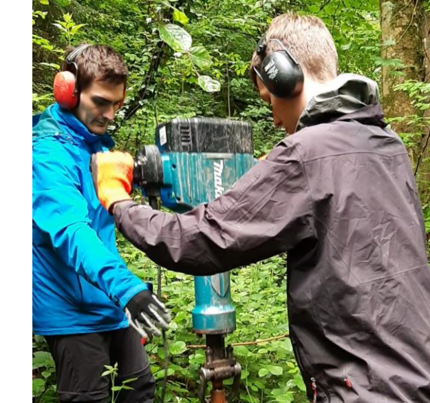
Drilling to refusal depth
