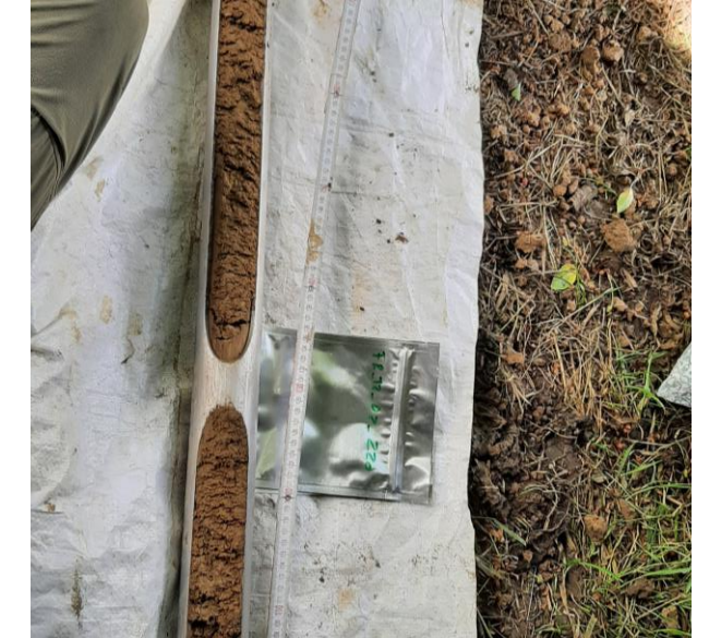
Sampling for Direct Vapor Equilibration
