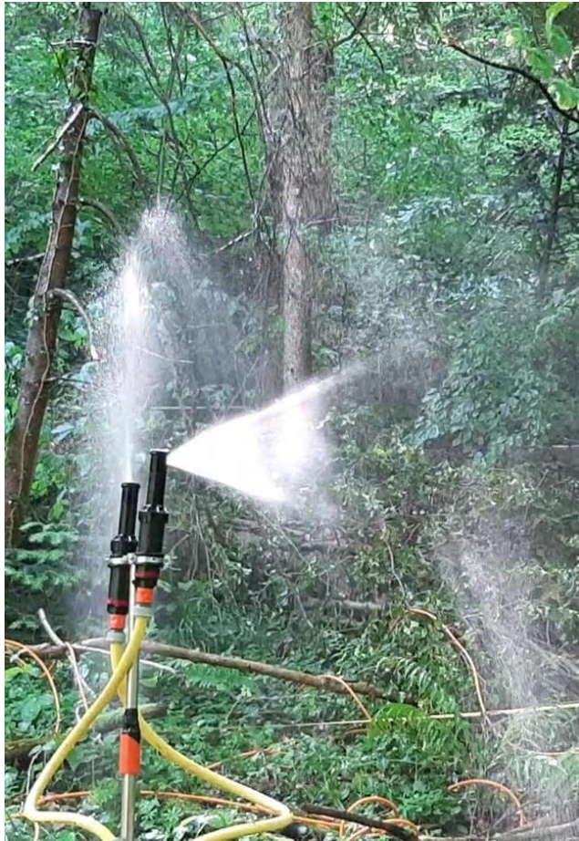
Sprinkled with 16 mm/h for 3h Deuterated water start 1.5 h
