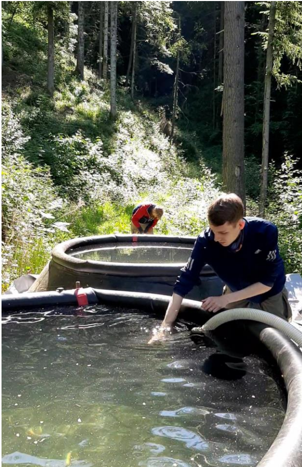
2x 4.5 m 3 Reservoirs 1x labeled \delta^2\text{H} to +220 ‰
