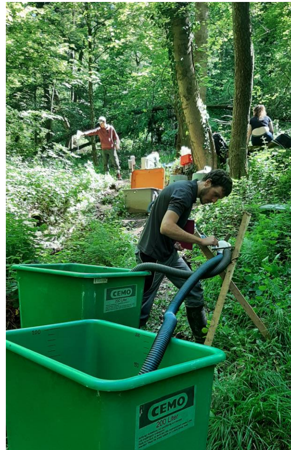
Continuous outflow monitoring
